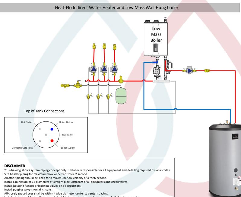
Install minimum of 6 pipe diameters of straight pipe upstream and downstream of all closely spaced tees. Differential pressure bypass valve prevents flow noise under partial load conditions (some zone valves closed). Set differential pressure bypass valve to delta P of distribution system with all zones open +1 psi.
